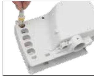
2. Unplug the cable contact from the hand control.
