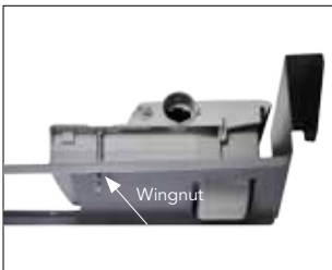
3. Unscrew the wingnut on the bottom that keeps electronics. Remove the screw.
