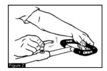
When the Quick-Up aid is used for moving, at least two of the wheels on the bed lift must always be locked.
